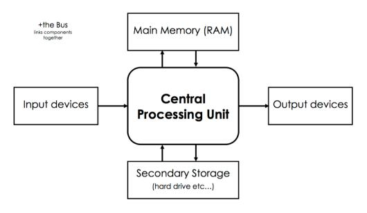
The wires connecting each part together are called the Bus.
